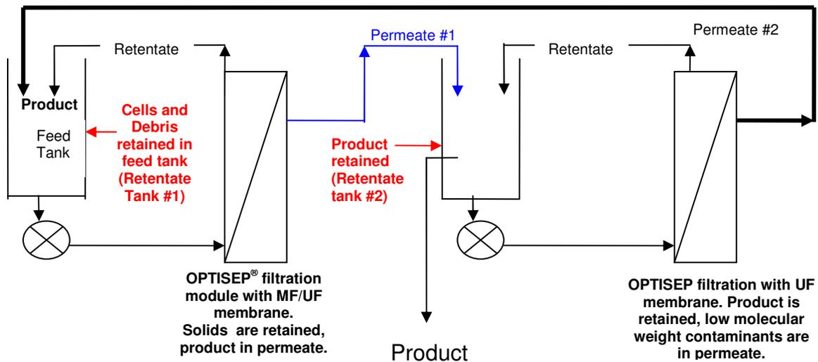
**Figure 1: Set-up for a simultaneous process**
