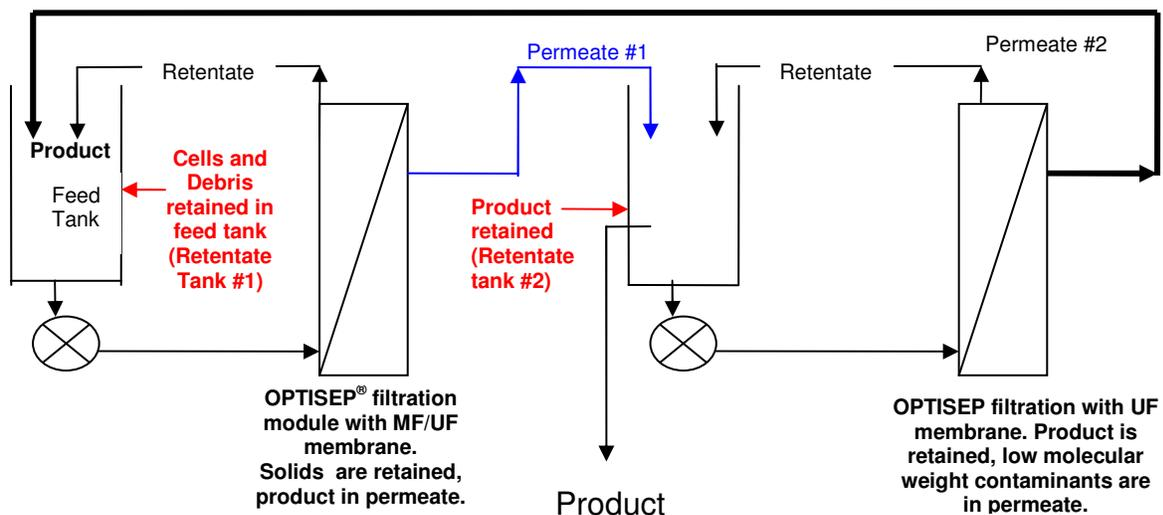
**Figure 1: Set-up for a simultaneous process**
